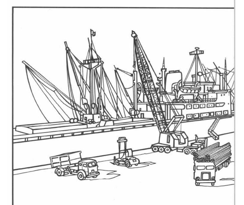
Cargo is handled at the Port in different ways. It is moved to the dock or loaded on a truck by a **fork lift** or **small crane**. A giant **container crane** lifts containers on and off the ship. Containers are large, strong boxes that hold all kinds of cargo in them. There are even special containers for automobiles, animals, liquids and other commodities. How is cargo handled in your Port?
